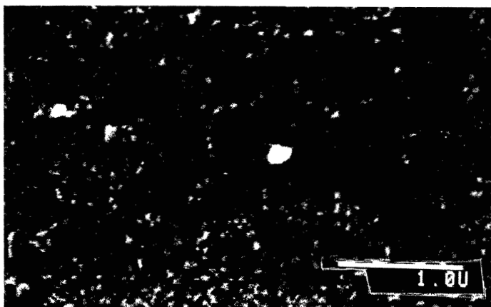
Figure 1: Electron micrograph of a PEI/PVP microfiltration membrane (top view of the membrane surface). The membrane was heat treated. Maximal pore size 0.05 \mu\text{m} .
